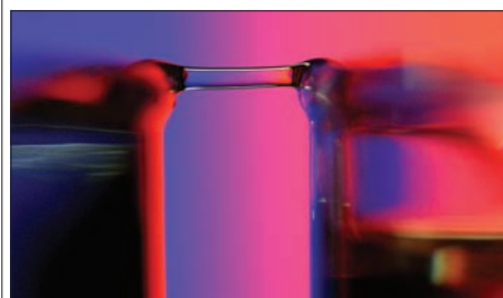
A bridge of water forms between two beakers. (Courtesy Fuchs/Woisetschläger.)
