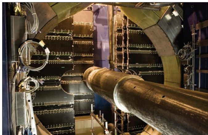
Fig. 4. Tracking stations 4 and 5, with the overlapping slat structure. (Courtesy Aurélien Muller for CERN.)
